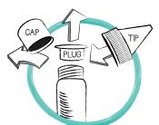
Uncap the tube. Remove and keep the protective plug. Then, twist on a tip.
